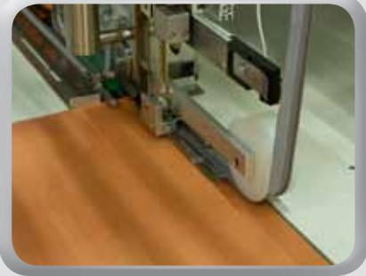
Special guiding devices are available for attaching zipper to material edge.
