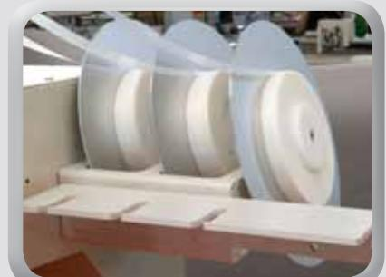
Adhesive tape spools are easily changed and remaining capacity is visible.
