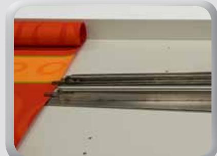
Material clamps hold the fabric in position during operation and avoid shrinkage on polyester based materials.
