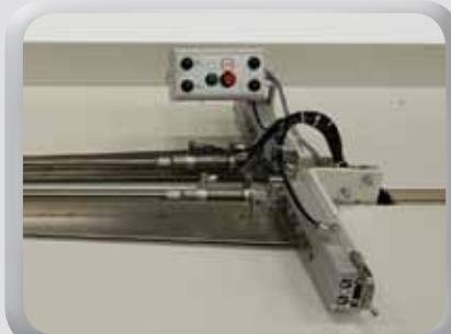
Optionally, an electrically adjustable clamp is available which, after entering the awning dimension, automatically travels to the position corresponding to the length of the fabric. This shortens the handling time by the operator.
