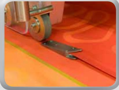
Option of automatic feeding apparatus for overlapping seams. With hemming guide from above, and overlap guide from below the appropriate guide is automatically positioned to minimize handling even further.
