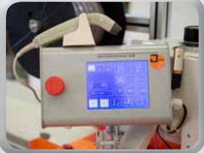
User friendly touch screen allows direct entry of machine parameters. Material specific settings can be easily stored and recalled.
