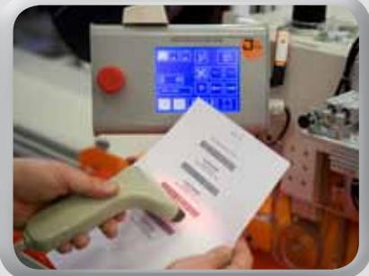
Optional barcode interface for reading setup and order parameters from work order. Connection to customer's network available.
