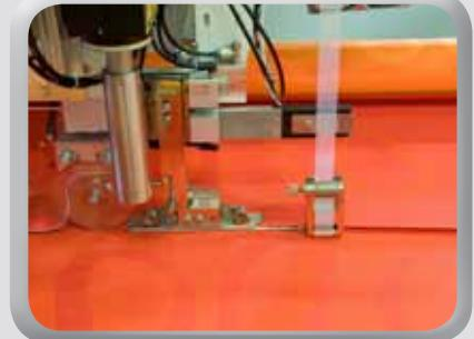
Application specific guiding devices are used to provide accurate seam and hem operations. Quick change device reduces change over time.
