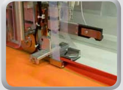
With the double hemming device option, the upper guide moves left / right as required for the side hems – no need to change guiding device.
