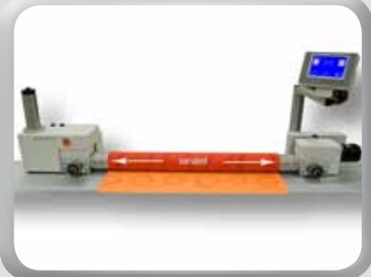
Optionally, a winding device for the seamed fabric panel is available. By means of the clamping jaws, the start and the end of the fabric panel is clamped and wound up under slight tension. Wrinkles and damage that can result from manual winding are thus avoided.
