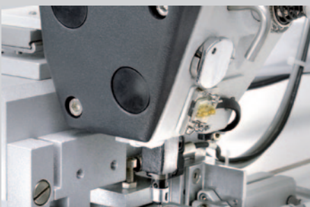
Upper thread monitor (standard on all machines) Thread clamp (option on -23/xx)
