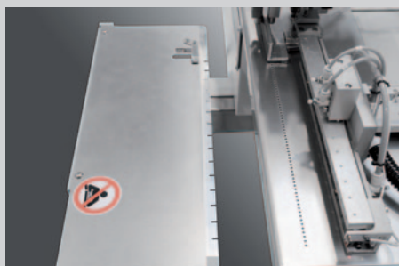
Larger feed table for double-pointed darts (Option on -23/01, -23/02)
